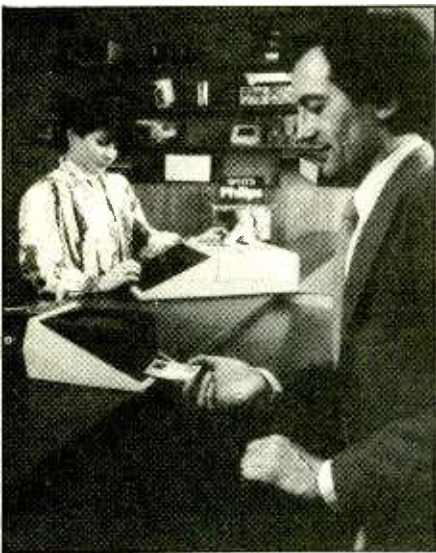
The electronic chequebook, the same size as a credit card contains a microprocessor and an e.p.r.o.m. The customer inserts it into a terminal while the assistant enters the transaction. The price is deducted automatically from the card (and from the customer's bank account!).
