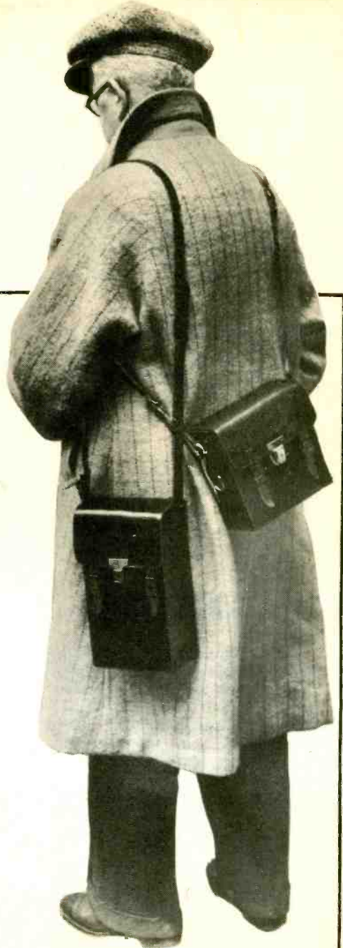
German Agentenfunk (Afu) transmitter in two cases, one for the batteries.
