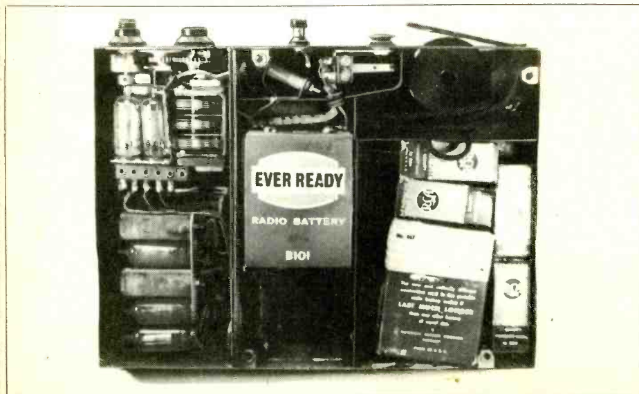
Special Communications briefcase receiver, using 1.5V valves and layer batteries, about 1943-4.
